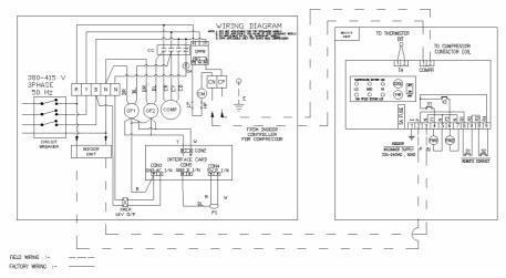
Figure 3. Wiring details DERVDX units
