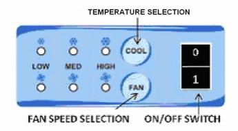
Figure 4. Controller display
