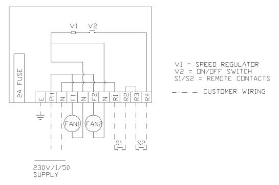
Figure 2. Wiring details DERV units
